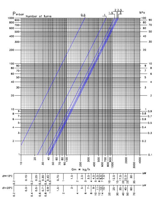
The preset positions are determened with the number of opening turns of the manual valve from the fully closed position.
