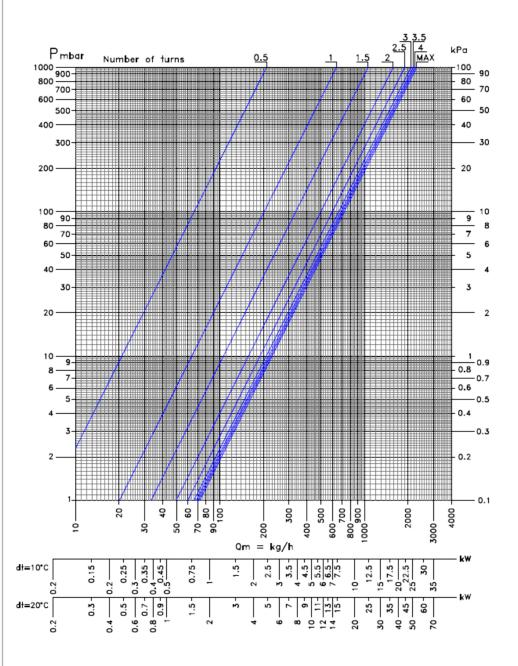
The preset positions are determened with the number of opening turns of the lockshield valve from the fully closed position.
